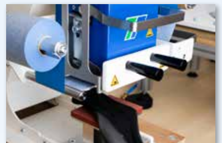
Printing with special heat seal ribbon
