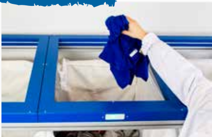
Light sensor frame to confirm where each item should go
